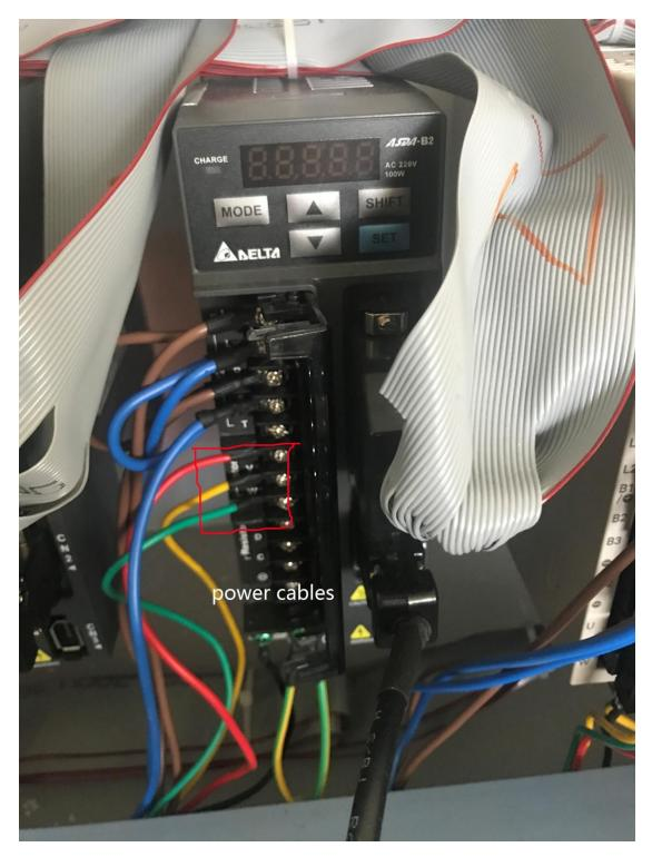
2. The cables are marked U, V, W. And the driver is marked Z1 or U1,Z2or
