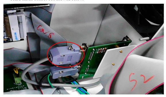
2. Plug out cable connector from communication board outside control box showed below.
